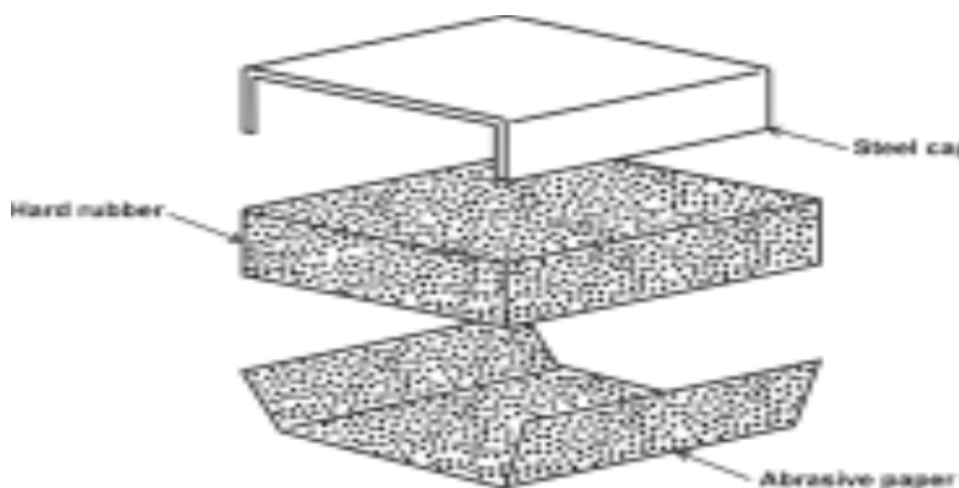
Fig. 1 – Example of pad rubber
